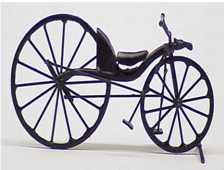
A Scottish blacksmith named **Kirkpatrick Macmillan** made the first mechanical bicycle in **1839**. It was driven by pressing down the treadles that moved up and down and turned the back wheel. On seeing someone ride velocipede he decided to make one for himself and ended making a tremendous change by adding paddles to it.
